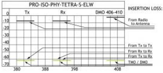
The built-in high-pass filter attenuates large signal interference and harmonic from radiosystems below 174 MHz.
